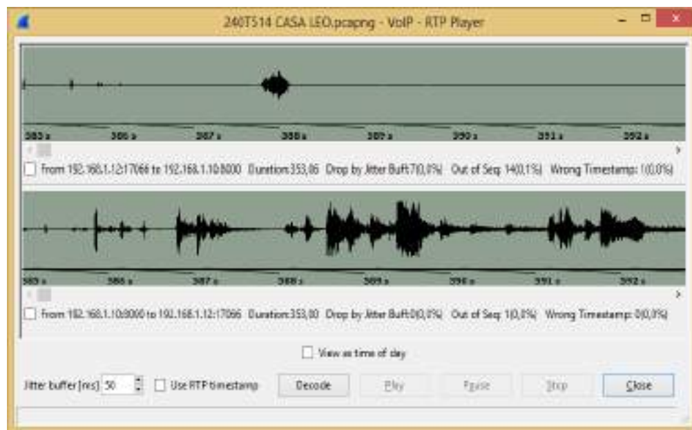
Figure 9. Decoding a VoIP call
